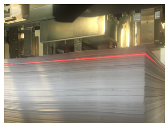
Laser pointer for pile surface equalizing
