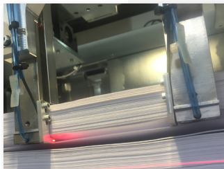
Physical check for "Correct Count" with optic fiber
