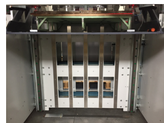
Motorized pile-aligner system with sensors
