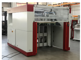
Delivery with automatic stacker
