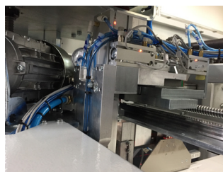
Linear movements on balls recycling guideways.
